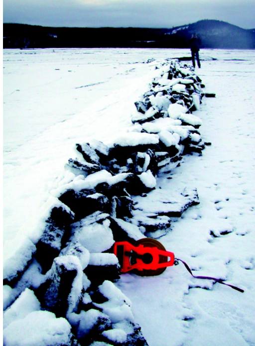
Figure 6. Lateral movement drove the crust down-slope where surface crust ( \sim 0.3 m thick) was rafted on a liquefied layer. In low-areas (here, a return channel) collision of two crusts resulted in between 3.8m and 4.3m of shortening (near SASW Site 588-TET). The tape measure handle is 15cm wide.
