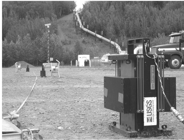
Figure 4. The preferred method of SASW testing uses a continuous harmonic-wave source produced by a low-frequency computer-controlled electromechanical shaker (device at right) and multi-sensor linear seismometer arrays (2-sensors on the left). This site is 600-PS11, at Trans Alaska Pipeline, Alyeska Pump Station 11, Glennallen, Alaska.
