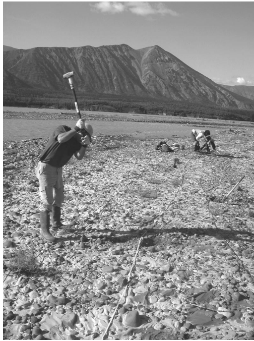
Figure 3. Hammer source SASW testing at site 583-NAB on the Nabesna River, a non-liquefaction site.
