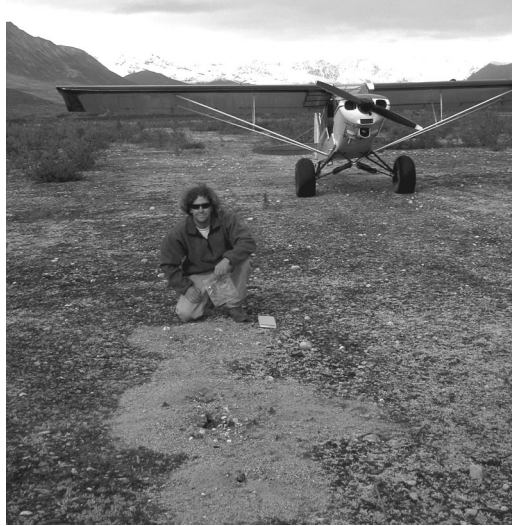
Figure 17. Sand boils in the upper Susitna River valley south of the Susitna Glacier terminal moraine.
