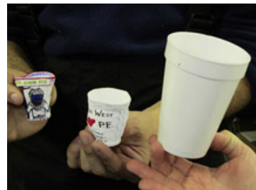
A closeup view of Mark's cups, with full-size cup on the right for scale. Although the lefthand cup went nearly 4 times as deep as the cup in the center, it did not shrink 4 times as much. We speculate that at a certain depth, all the air has been pressed out of the Styrofoam and no further shrinking takes place as the cup keeps going down. (We are too far north to access the Internet to check on this hypothesis!). Click image for larger view. Credit: Helen Gibbons, USGS/ECS Project.
