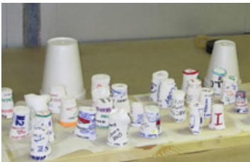
A closeup view of Mark's cups, with full-size cup on the right for scale. Although the lefthand cup went nearly 4 times as deep as the cup in the center, it did not shrink 4 times as much. We speculate that at a certain depth, all the air has been pressed out of the Styrofoam and no further shrinking takes place as the cup keeps going down. Click image for larger view. Credit: Helen Gibbons, USGS/ECS Project.
