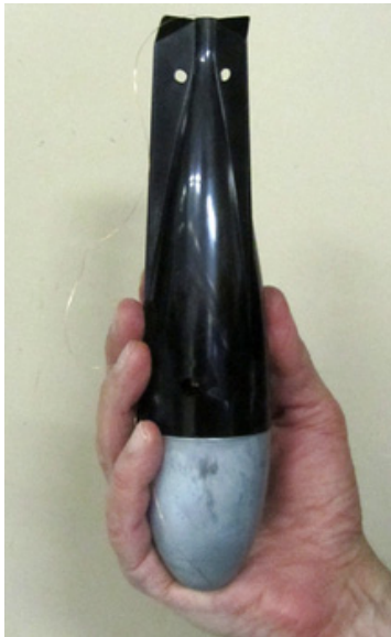
Expendable bathythermograph (XBT) probe (a faulty one that was never launched). As this torpedo-shaped probe falls through the water, a thermistor in the tip continuously measures temperature. The thin wire that passes data back to the ship is barely visible on the left. Click image for larger view. Credit: Helen Gibbons, USGS/ECS Project.
