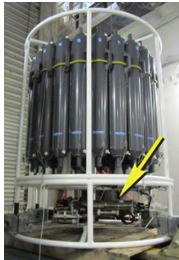
Package of CTD electronics and sensors (arrow) is mounted below a ring of water-collecting bottles. Click image for larger view. Credit: Helen Gibbons, USGS/ECS Project.
