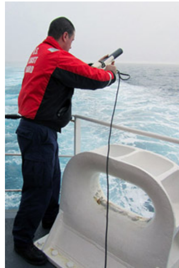
MST3 Daniel Purse prepares to launch an XBT off Healy's stern. The black wire connects the launcher to a computer in the Aft Conn, a control room overlooking the stern of the ship. Click image for larger view. Credit: Helen Gibbons, USGS/ECS Project.
