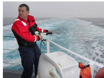
The probe is in the water and falling toward the seafloor. A thin wire (not visible in this photo) connects the probe to the launcher. With his left hand, Dan holds the connecting wire away from the railing while he watches MST3 Marshal Chaidez in the Aft Conn for the signal that the probe has reached the seafloor. At Marshal's signal, Dan will snap the connecting wire and bring the launcher back inside the ship. The probe stays on the seafloor. Click image for larger view. Credit Helen Gibbons, USGS/ECS Project.
