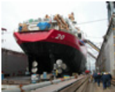
Sep 5 Log The box-like shape of Healy's hull contributes to her stability. In this photo of Healy in dry dock in 2004, you can see the nearly straight sides of the hull. Credit: Captain William Rall, U.S. Coast Guard.
