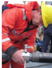
Aug 11 Log Andy fits a cutting device onto the plastic core liner of the piston core, which has been pulled partway out of the metal core barrel. Credit: Helen Gibbons, USGS/ECS Project
