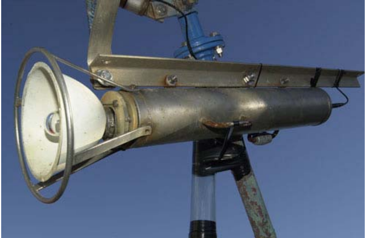
Figure 5. Benthos underwater strobe mounted on tripod frame. The reflector is painted with white antifouling paint to discourage biological growth. See figs. 2 and 3 for overview of frame.
