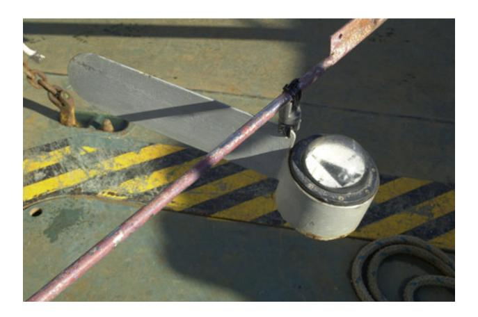
Figure 6. Compass and vane assembly mounted in the field of view of the camera. The vane orients in the current and shows the flow direction when the pictures are taken; the compass indicates magnetic north (16 degrees west of true north at Site A).
