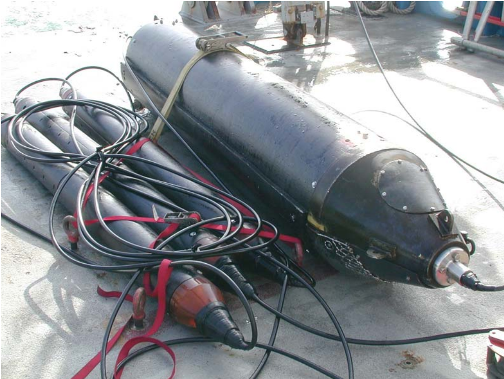
Figure 1 A photograph of the towed EM system on deck. The system consists of a transmitter (large cylinder at right) connected to the ship by a 0.680 conducting cable. Three receivers (smaller cylinders) to behind the transmitter at separations of 4m, 13m and 40m and provide information to depths of about 20m subsurface.
