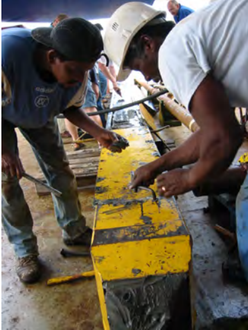
Figure 46. Top panels being removed from a box corer. Notice the pyramid shape to the recovered sediment at the bottom of the core.
