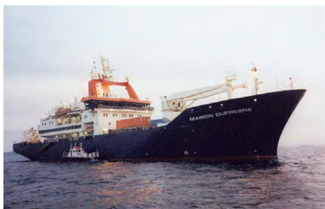
Figure 1. RV Marion Dufresne is 120.5 meters in overall length and is 20.6 meters in beam amidships. It has a draft of 6.95 meters and displaces 10,380 tonnes. Coring operations are conducted using the starboard stern A frame.
