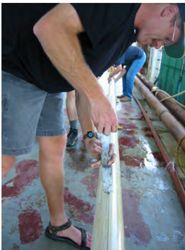
Figure 19. Gas sample being collected from a hole drilled in a Calypso PVC core liner.
