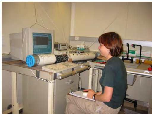
Figure 34. Thermal conductivity measurements were performed on whole-round core sections using a needle probe after the sediment temperature equilibrated.
