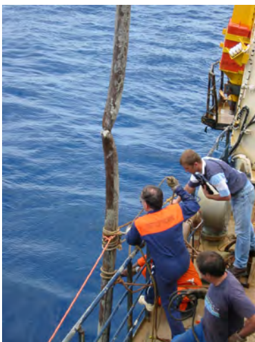
Figure 42. The core barrel would actually break if enough stress was placed on it during the coring and recovery process.
