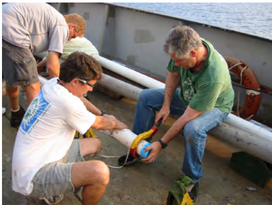
Figure 30. Whole-round samples, 10-centimeter to 25-centimeter long, were cut from the ends of core sections every 1.5 meters.
