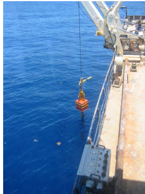
Figure 3. Calypso piston corer ready to be lowered. Notice the yellow-colored trigger arm attached to the main cable above the weight stand. The main corer is held in position until a weight suspended from the trigger arm contacts the sea floor. As tension on the trigger arm is reduced, the main corer is released and is driven into the sea floor by the massive weight stand.
