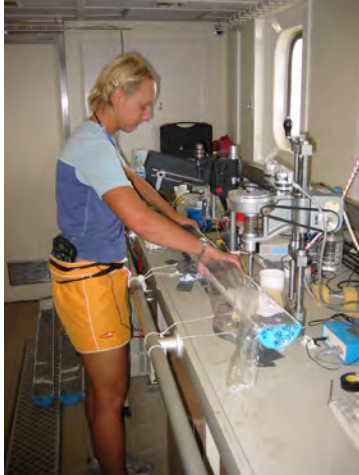
Figure 39. A suite of physical property measurements were made on the working half of the cores. A mini-vane shear machine is located in the foreground.
