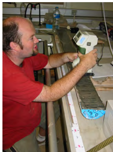
Figure 37. Sediment color on the archive-half split core was recorded with a spectrophotometer.
