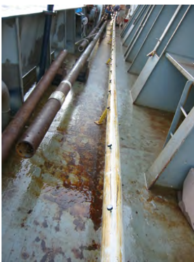
Figure 22. Digital thermometers were inserted at 1-meter intervals down core.
