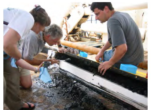
Figure 53. Sediment from a box core being placed into a sample holder that will be used to squeeze pore water from the sediment pore spaces.
