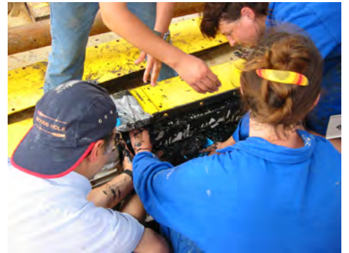
Figure 51. Removal of a U-channel from a box core.
