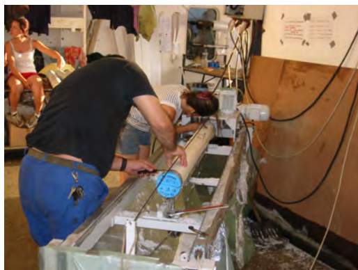
Figure 35. The core was longitudinally split after whole-round sections were removed.
