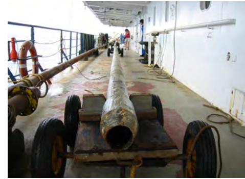
Figure 6. Recovered Calypso corer ready to be dismantled.
