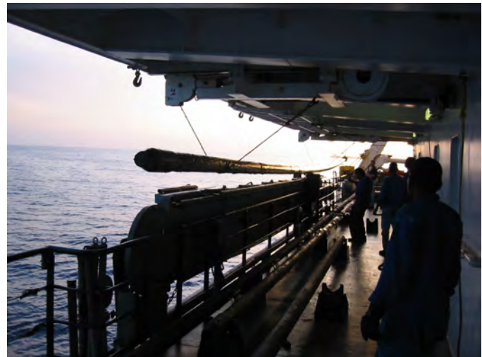
Figure 4. Recovery of a Calypso piston corer.
