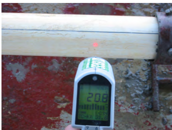
Figure 16. The surface temperature of the core liner was measured with an infrared sensor after it was removed from the metal core barrel.
