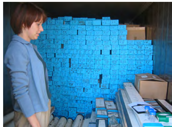
Figure 33. Core sections were refrigerated at approximately 4 degrees Celsius during storage.
