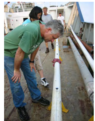
Figure 21. Thermometers were monitored to determine low thermal anomalies suggestive of gas hydrate dissociation.
