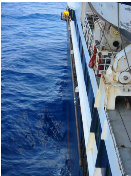
Figure 2. Calypso piston corer about to be pivoted into a vertical position for coring.
