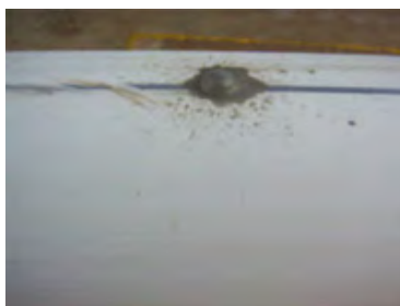
Figure 25. Click here to view video* of gas being extruded from holes drilled in the core liner.
