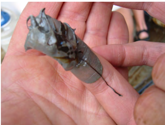
Figure 56. Hydrocarbons recovered in box core MD02-2563C2. Notice the filament-like, viscous nature of the hydrocarbons.
