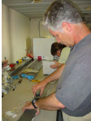
Figure 40. The working half of the split cores was subsampled for water content and other properties. A Torvane test is being performed in the foreground.
