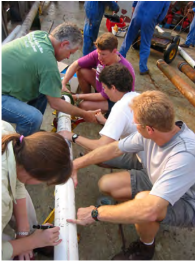
Figure 29. After the PVC core liner was removed from the metal core barrel, it was labeled and cut into 1.5-meter lengths.
