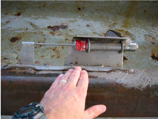
Figure 14. Side view of a heat-flow temperature sensor.
