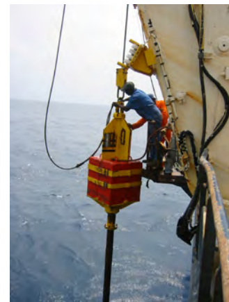
Figure 8. Weight stand used to drive the core barrel into the sea floor.
