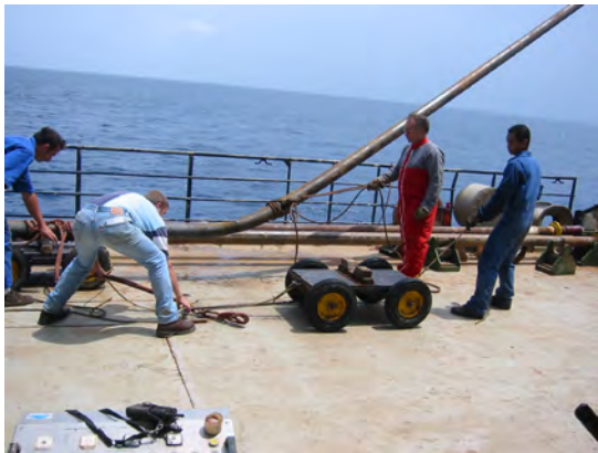
Figure 41. Bent core barrels required special handling procedures.
