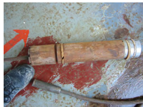
Figure 9. A critical component of a piston-coring system is the piston that theoretically remains near the level of the sea floor during sediment penetration by the core barrel. The vacuum that develops between the bottom of the piston and the sediment surface helps overcome the frictional forces between the cored sediment and the internal wall of the barrel liner.
