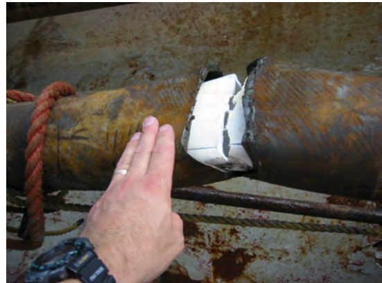
Figure 43. Although most of the core barrel broke during the coring operation, enough strength existed in the remaining barrel and liner to enable retrieval of the core.
