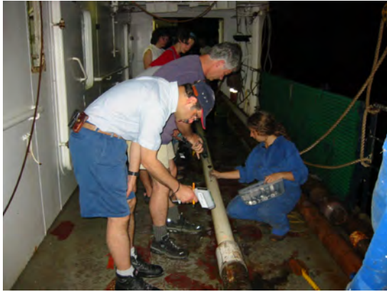
Figure 17. Immediately after the PVC core liner is pulled from the metal core barrel the surface temperature was determined with a hand-held infrared thermal sensor.
