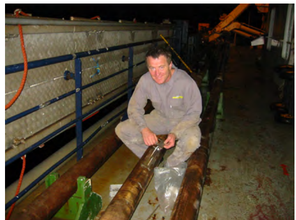
Figure 13. Installation of a heat-flow sensor onto an outrigger welded to a gravity corer.
