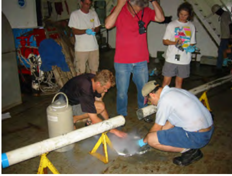
Figure 59. Removal of core sections containing gas hydrate was based on low sediment liner surface or internal sediment temperature anomalies. Samples were immediately placed in the liquid nitrogen Dewar shown next to the core.
