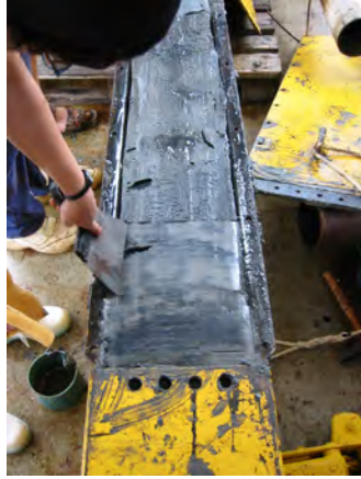
Figure 47. Sediment surface being scraped to enhance interpretation of stratigraphic features.
