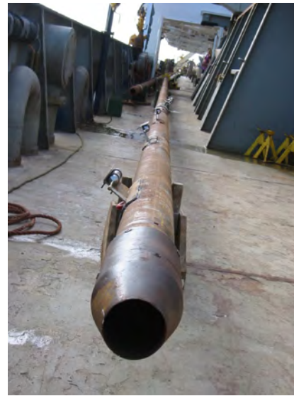
Figure 12. Gravity core with staggered outrigger heat-flow sensors.
