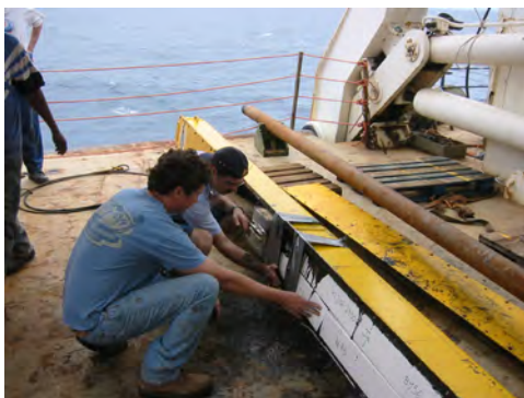
Figure 50. A box core on its side. Notice the styfoam plug at the top of the core used to stabilize the soft sediment surface.
