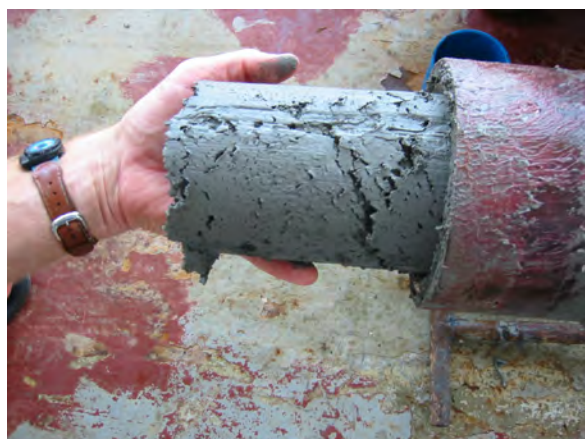
Figure 27. Occasionally gas expansion caused sediment to self extrude.
