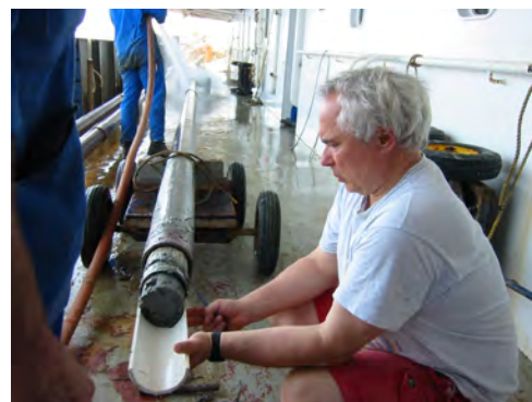
Figure 26. Sediment that “self-extruded” because of gas expansion sometimes needed to be collected on a half-round PVC liner.
