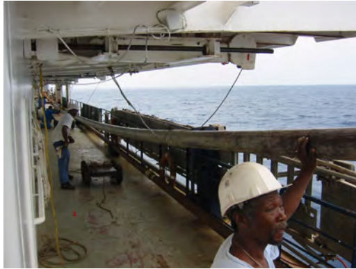
Figure 5. Recovered Calypso piston corer being lowered to the deck.
