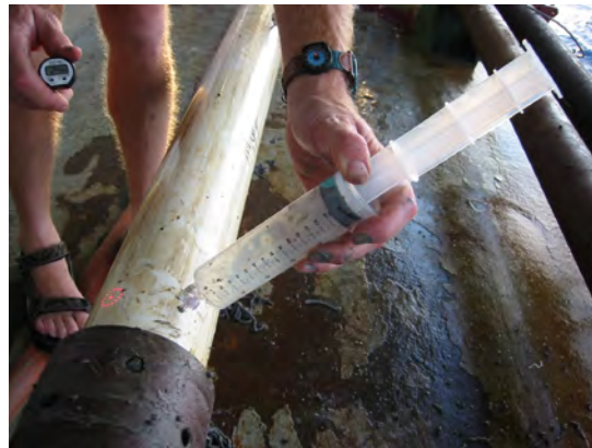
Figure 20. Syringe filled with gas to be later analyzed for isotopic composition.
