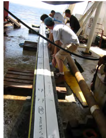
Figure 49. A box core about to be tipped onto its side.
