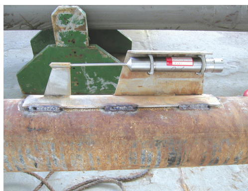
Figure 4B. A Micrel autonomous temperature sensor welded onto a gravity-core barrel. Because the sensor is fully self contained, there is no connector and no power switch. Dialog is performed using a reading pen connected to the serial port of a personal computer. Batteries and a data logger are contained in a 172-millimeter (mm)- long, 28-mm-diameter titanium cylinder. Two temperature probes are contained in a 130-mm-long, 4-mm-diameter titanium needle. The probe is located 60 mm from the core barrel. This distance ensures that it will take 1 hour for the heat generated by the friction of penetration to reach the needle probe. Probe temperature range: -2 to 35 degrees Celsius ( ^{\circ}\text{C} ); linearity: \pm 2 milli-degrees Celsius ( \text{m}^{\circ}\text{C} ); resolution: 0.6 \text{m}^{\circ}\text{C} ; stability: 20 \text{m}^{\circ}\text{C}/\text{year} ; repeatability: \pm 0.6 \text{m}^{\circ}\text{C} ; total measurement range: -2 to 75 ^{\circ}\text{C} ; maximum water depth: 6,000 meters (m).
