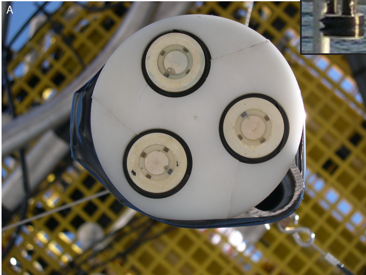
Figure 27. A photograph of acoustic transducers (A) on an Acoustic Backscatter Sensor (ABS) (B). The ABS transducers emit pulses of high frequency sound which are reflected by suspended sediments in the water column. The quantity of sound reflected back to the sensor is combined with instrument calibration information to derive vertical profiles of suspended sediment concentrations.
