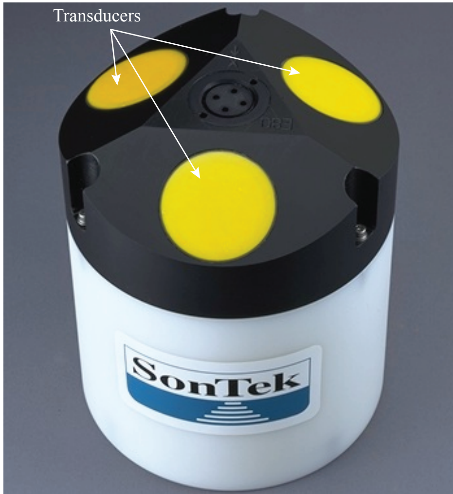
Figure 20. A photograph of a SonTek Argonaut-XR (Extended Range) Acoustic Doppler Profiler (ADP). The ADP's three transducers (yellow circles in the photograph) transmit and receive sound along acoustic beams. Because Doppler shift is proportional to the component of water flow along the beams, trigonometry can be used to convert the returned acoustic signal into eastward, northward, and vertical components of water flow. This photo is courtesy of SonTek.
