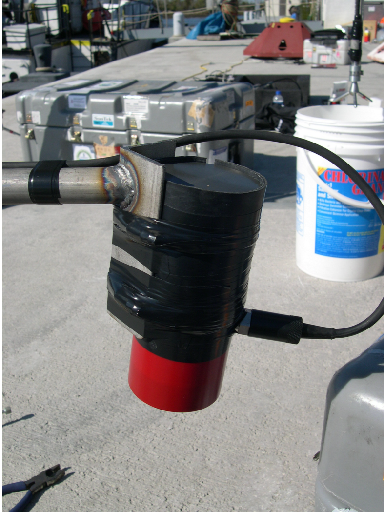
Figure 28. A photograph of the Imagenex 881A imaging sonar. The sonar emits beams of high frequency sound which reflect off objects and bedforms on the sea floor. The sonar was deployed at Site 6 from October 2003 through April 2004 and was used to observe sea floor bedforms (ripples).
