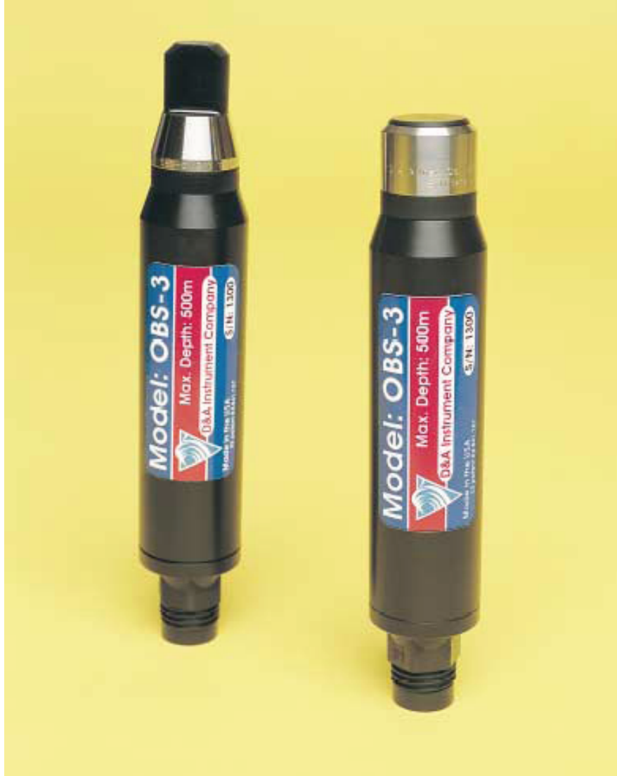
Figure 26. A photograph of D&A Instruments Optical Backscatter Sensors (OBS). The OBS emits a beam of infrared light that is scattered by suspended sediments in the water column. Suspended sediment concentration is derived by combining the quantity of light reflected back to the sensor with sensor calibration coefficients. This photo is courtesy of D&A Instruments.
