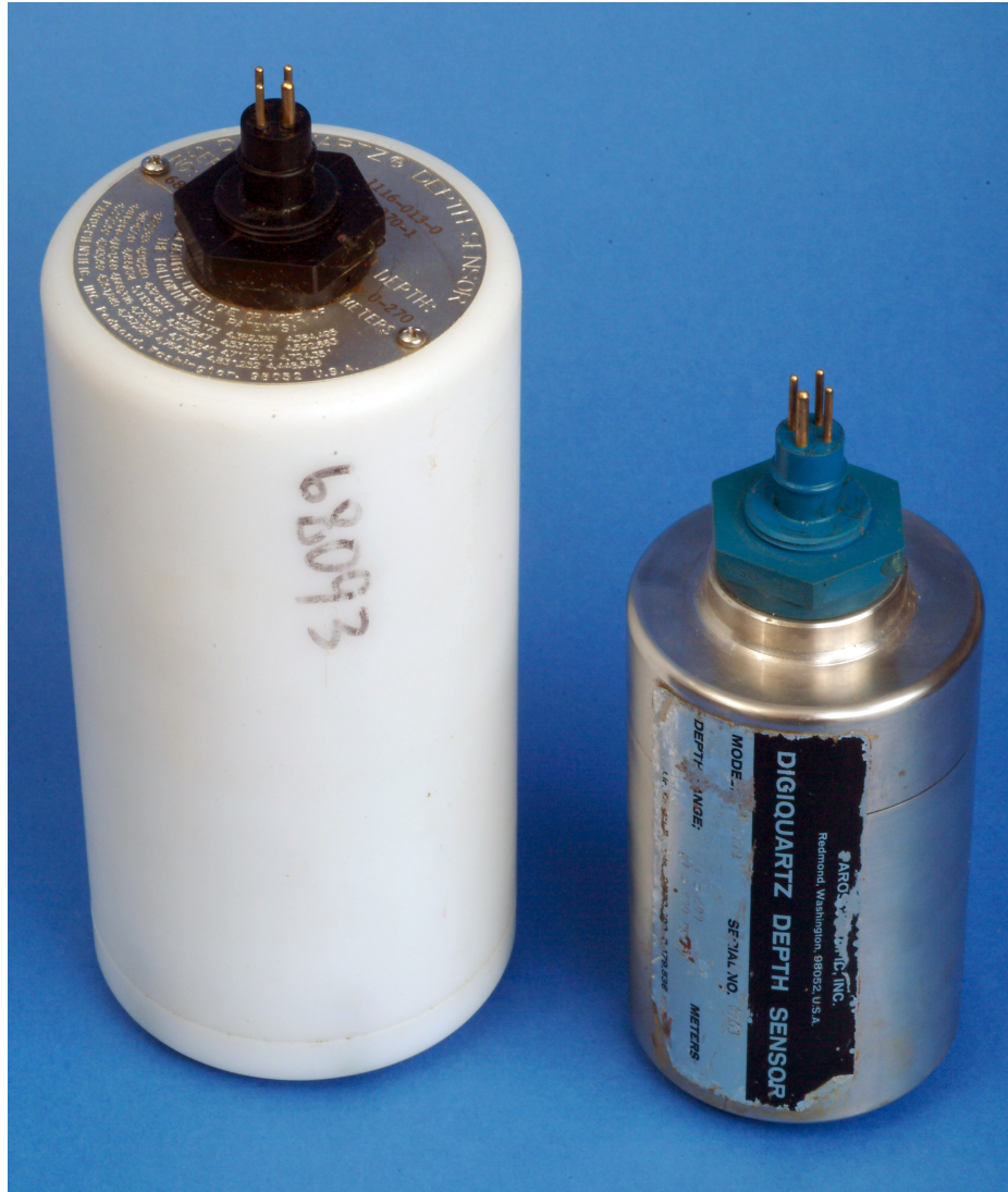
Figure 23. A photograph of Paroscientific Digiquartz® pressure sensors. The sensors measure pressure using special quartz crystal resonators. The frequency of oscillation of these resonators varies with pressure induced stress.
