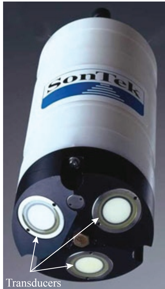
Figure 21. A photograph of a SonTek Pulse-Coherent Acoustic Doppler Profiler (PCADP). The PCADP measures water flow from the Doppler shift that occurs when scatterers, that are carried by the water, reflect paired acoustic pulses along three acoustic beams. PCADP measurements of water flow in along-beam regions as small as 1.6 centimeters offer increased spatial resolution over single acoustic pulse instruments (ie. ADCP). This photo is courtesy of SonTek.
