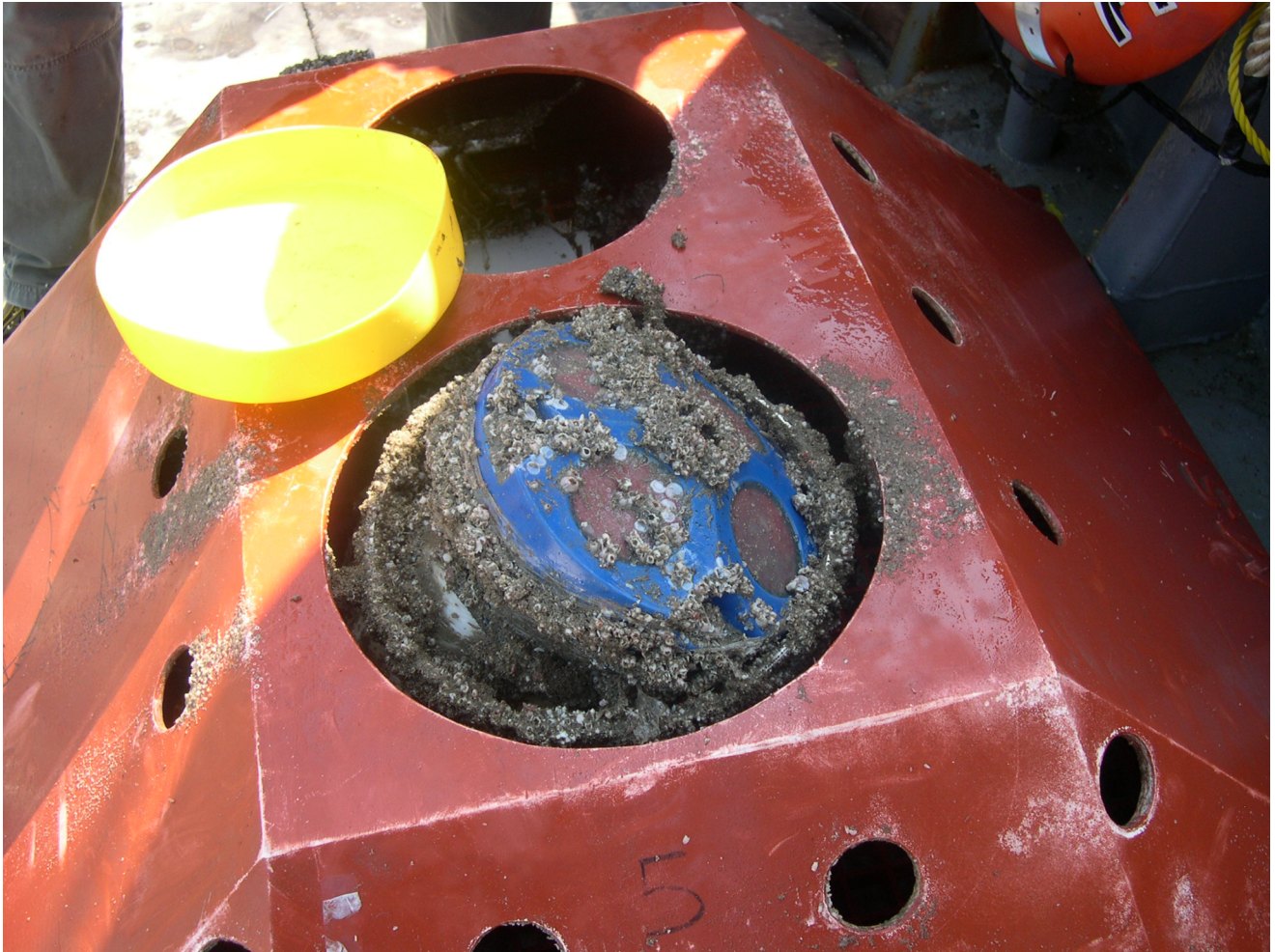
Figure 18. A post-recovery photograph of the ADCP deployed at Site 5. The ADCP was deployed in a TRBM. As seen in this photo, the ADCP became significantly tilted ( >25 degrees) while in the TRBM. Data from this ADCP could not be salvaged and is not included in this report.
