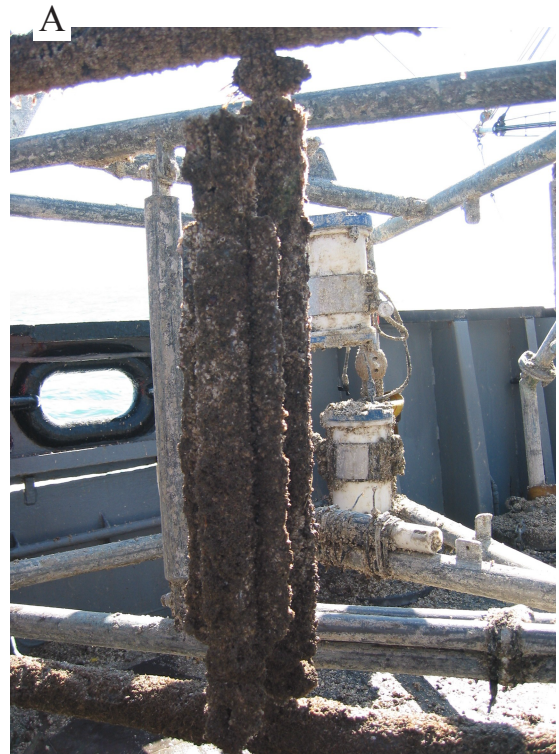
Figure 34. (A) A photograph of the tripod recovered from Site 3 at the end of the first deployment. All instruments experienced some biofouling. (B) A photograph of the ADCP mounted to the tripod shown in (A). Two of the transducers on the ADCP were biofouled (one significantly).
