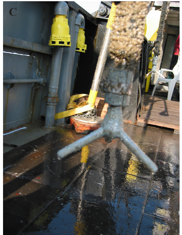
Figure 40. (A) Photograph of the tripod recovered from Site 6 at the end of the second deployment. Biofouling of the tripod surfaces and the surfaces of instruments was not significant. (B) Photograph of the ABS and (C) photograph of the ADV mounted to the tripod in (A).
