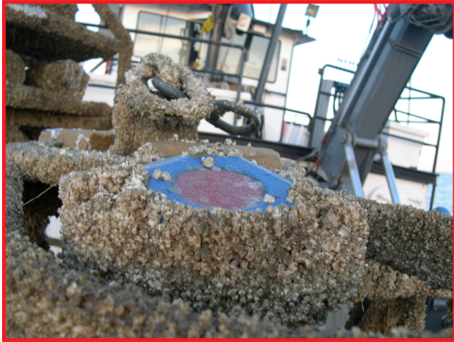
Figure 43. Photographs of the tripod and instruments recovered from Site 7B at the end of the first deployment. The tripod surfaces are significantly biofouled, as are the surfaces of all instruments on the tripod.
