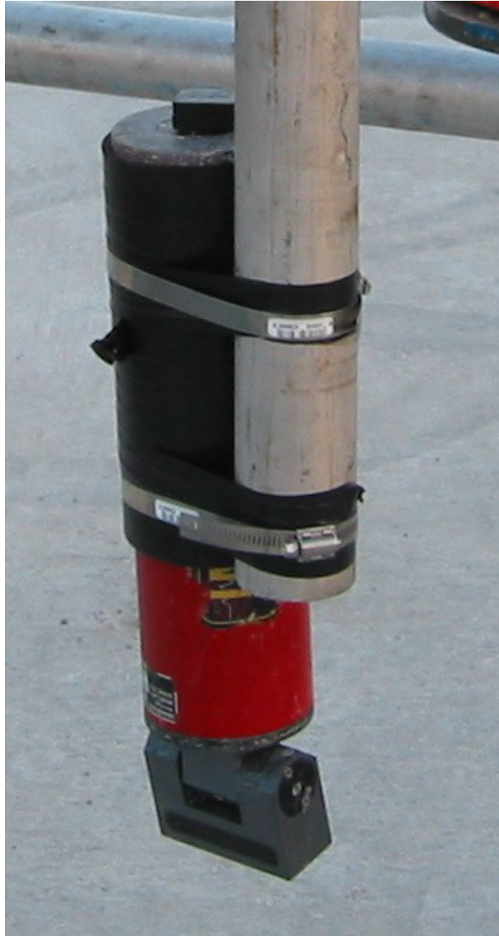
Figure 29. A photograph of the Imagenex 881 tilt-adjusting imaging sonar. The sonar emits beams of high frequency sound which reflect off objects and bedforms on the sea floor. The sonar was deployed at Site 7B from October 2003 through April 2004 and was used to observe sea floor bedforms (ripples).
