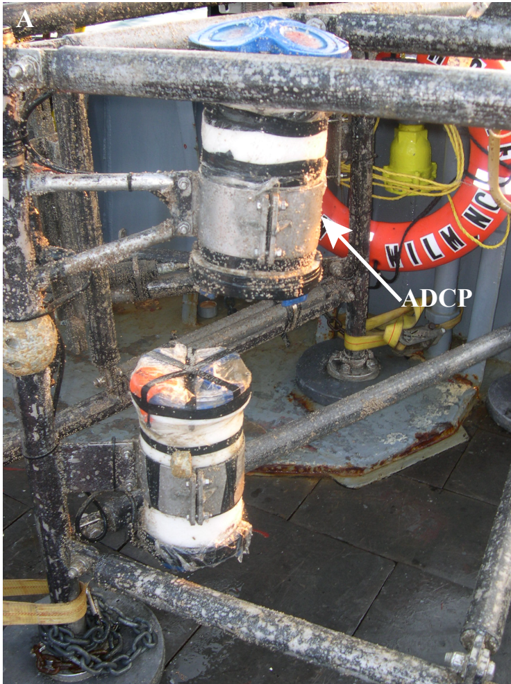
Figure 31. (A) A photograph of the tripod recovered from Site 1 at the end of the second deployment. (B) A photograph of the ADCP mounted to the tripod shown in (A). Both the ADCP and the tripod were significantly less biofouled during the second deployment.
