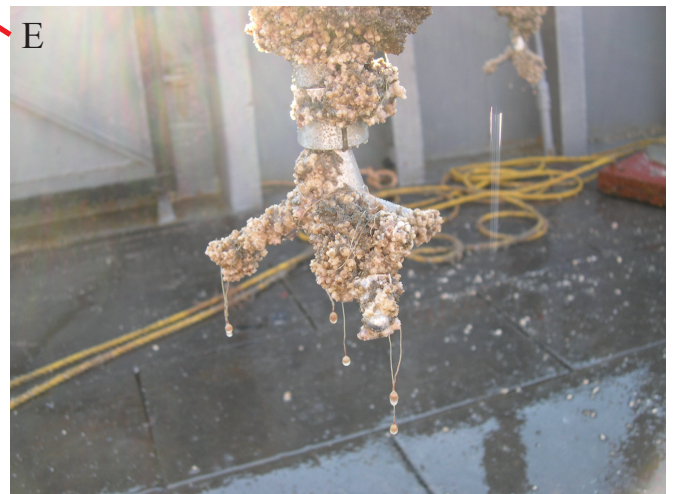
Figure 39. (A) Photographs of the tripod recovered from Site 6 at the end of the first deployment. The surfaces of the tripod and instruments are significantly biofouled. Photos of the barnacle-encrusted instruments are provided in (B) through (E).
