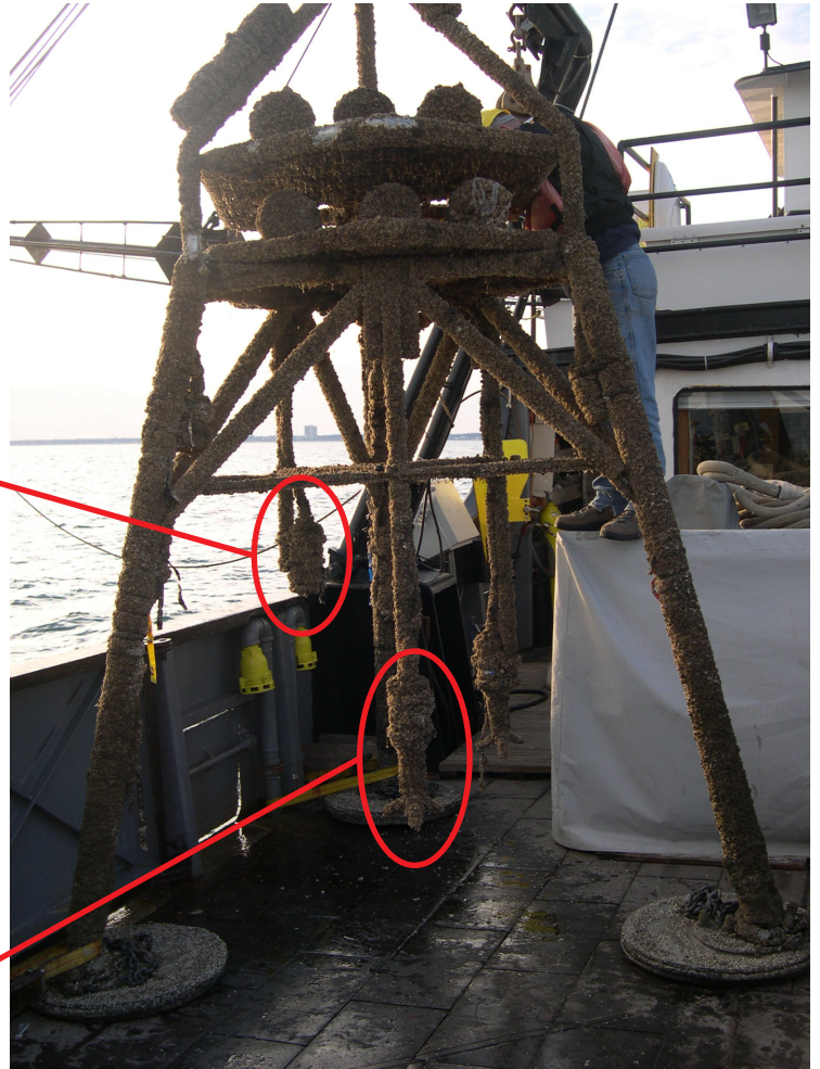
Figure 41. A photograph of the tripod recovered from Site 7A at the end of the first deployment. The surfaces of the tripod and all instruments on the tripod were heavily encrusted with biofouling.
