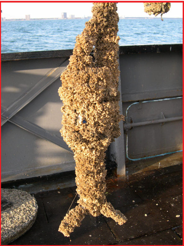
Figure 41. A photograph of the tripod recovered from Site 7A at the end of the first deployment. The surfaces of the tripod and all instruments on the tripod were heavily encrusted with biofouling.
