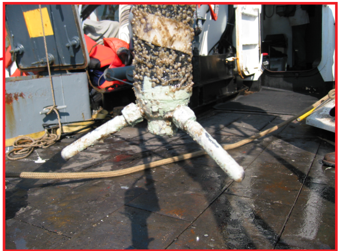
Figure 42. Photographs of the tripod and instruments recovered at Site 7A at the end of the second deployment. Biofouling was not as significant during this deployment.
