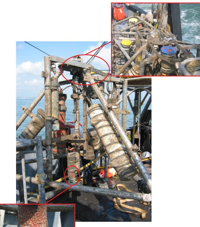
Figure 44. Photographs of the tripod and instruments recovered from Site 7B at the end of the second deployment. Biofouling was not very significant during this deployment.
