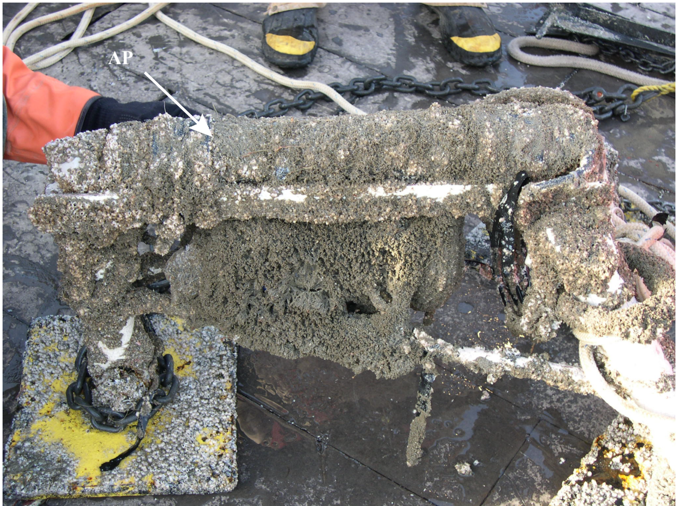
Figure 45. A photograph of the tripod recovered from Site 8 at the end of the first deployment. The surface of the tripod and the surface of the AP are heavily biofouled.
